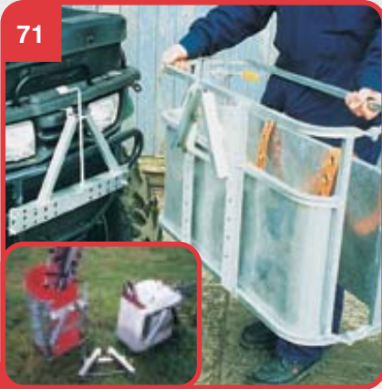
71 S300 'A' FRAME the basis of the System 30 can be supplied as a kit or as part of this S310KC Calf Crate product. The adjustable frame and installation kit ensure correct mounting. A ¼ turn spring catch releases equipment to be lifted off.
