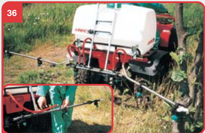
36 OBS BOOMS range from 1.5m (3 nozzle) to 3.5m (7 nozzle) in width, 3 and 4 nozzle booms are rigid with single breakback clutch, 5,6 & 7 nozzle booms are folding with breakback clutches on each wing to ensure no damage when working close to fences or hedges etc. All nozzles including hedgerow nozzle incorporate individual switch off and anti-drip facility.
