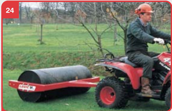
BR120/150 BALLAST ROLLERS come in two widths 1.2m or 1.5m. Liquid weight can be adjusted to suit ground conditions, features include large 560mm dia heavy wall section drum for easy towing, 50mm dia axle, long life sealed bearings and adjustable rear scraper.
