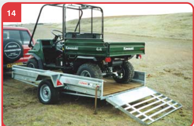
14 LT706 Purpose built to carry larger ATVs e.g. Kawasaki Mule, 4x wheel Polaris Rangers or similar weighted equipment. Body size 2970 x 1550 x 300mm, other features: heavy duty loading ramp, auto reverse brakes, parking brake, jockey wheel and prop stands.
