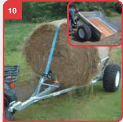
10 LBT TIPPING BALE TRAILER designed to self-load, carry and tip hay and straw round bales. Ideal for equestrian units and livestock farms, maximum load 600kg. Inset shows trailer body version available to carry and tip bales and a wide range of materials.
