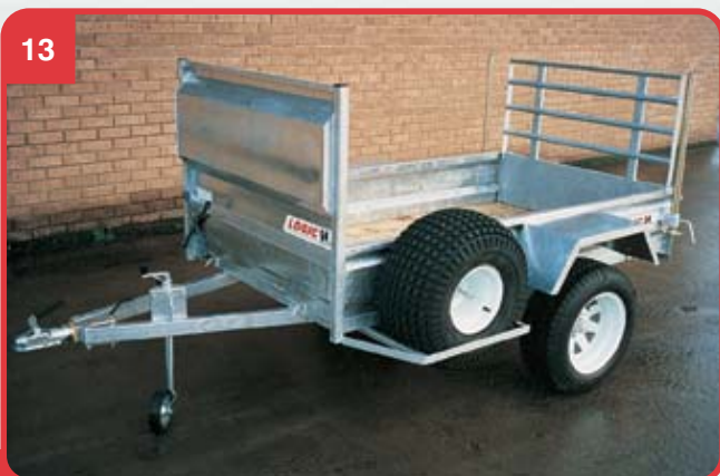
13 EBT300/400 TRAILER developed specifically for the needs of electricity companies. Used to carry an ATV to the site then behind the ATV to carry equipment. Work rates have been improved and land damage compensation reduced. EBT300: 2020 x 1160 x 300mm; EBT400: 2520 x 1160 x 300mm. Options: rear prop stands, jockey wheel and WT810 flotation tyres.
