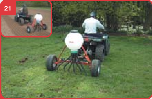
LSS100E SEED SPIDER™ is a precision seeder designed for sowing various seeds eg. Grass seed mixtures. Its electronic metering system can handle a wide range of seed types. Hardened chisel point openers allow direct seeding in grassland, ideal for patching worn paddocks etc. Inset shows LSS100E sowing an arable crop. They are easy to use and have workrates of up to 1 Ha/hr.
