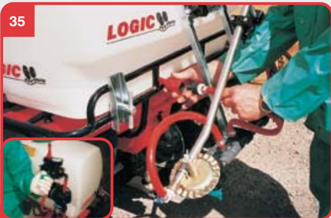
35 QUICK ATTACH design features include the use of two large hand tightened "T" bolts which quickly secure the OBS sprayer to most ATV carrying frames. Snap couplings are used on boom or hand lance hose connections. Inset shows OBS CONTROLS , offering easy access to on/off switch, pressure regulator, spray/agitate lever and in-line filter.
