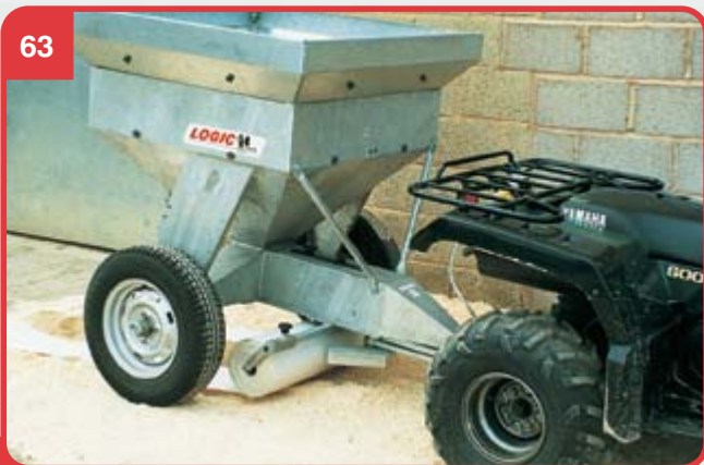
63 LCF160 CHICK FEEDER mechanises the time consuming job of laying feed onto paper in poultry houses. Features include hopper capacity up to 500kg, adjustable paper holder up to 1000mm width and 12 volt electrical remote on/off control allowing use with various vehicles, eg. Bobcat. One person can prepare a shed with 1500kg of feed in approximately 20 minutes.
